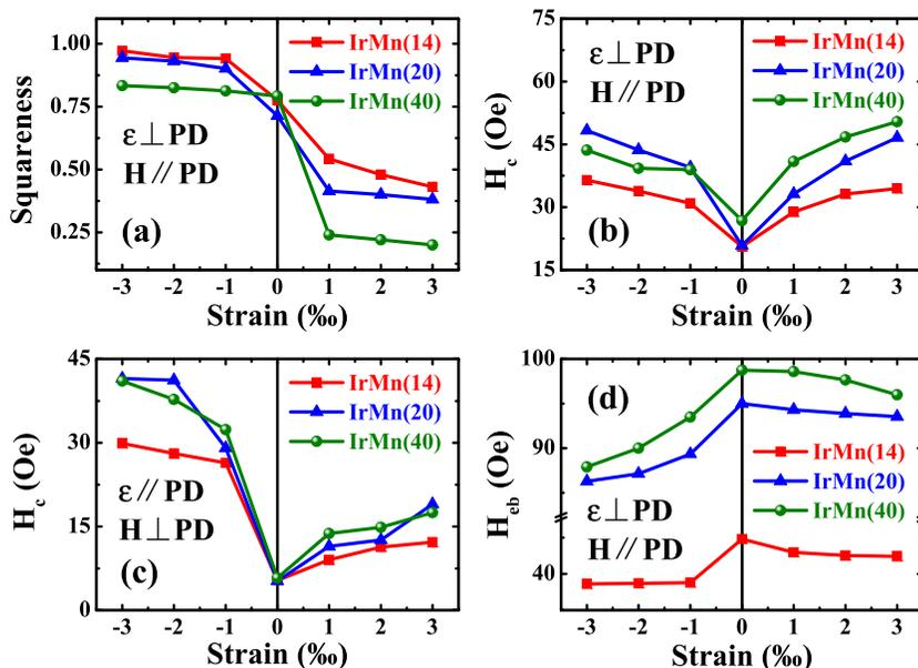
FIG. 3. The applied strain dependence of (a) loop squareness, (b)  $H_c$ , and (d)  $H_{eb}$  for  $H$  parallel and  $\varepsilon$  perpendicular to the PD, and (d)  $H_c$  for  $H$  perpendicular and  $\varepsilon$  parallel to the PD in FeGa(10 nm)/IrMn( $t_{\text{IrMn}}$ ) bilayers with different  $t_{\text{IrMn}}$ .
