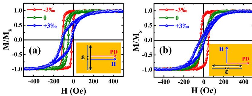
FIG. 2. The applied strain dependence of magnetic hysteresis loops for FeGa(10 nm)/IrMn(20 nm) bilayers with magnetic field (a) parallel and (b) perpendicular to the PD. The compressive and tensile strains are applied perpendicular or parallel to the PD, as shown in the insets of (a) and (b), respectively.
