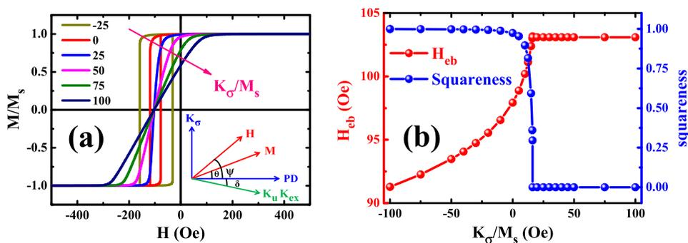
FIG. 4. (a) Calculated hysteresis loops under various stress-induced magnetic anisotropy fields of  $K_{\sigma}/M_s$  for the flexible exchange biased bilayer with H parallel to the PD using a modified Stoner-Wohlfarth model. The geometries of the magnetic anisotropies and the applied stresses are shown in the inset of (a). (b) The calculated loop squareness (blue line) and  $H_{cb}$  (red line) as a function of  $K_{\sigma}/M_s$ .
